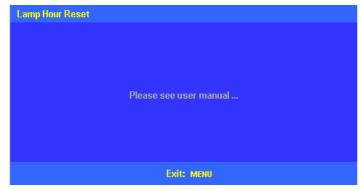
Press the cursor keys through following sequence to reset Lamp hour: down → → up ▲ → left ◄ → right ▶
